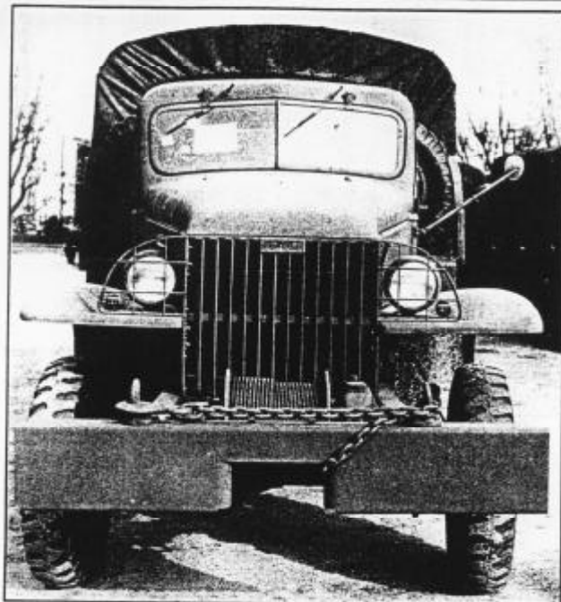
Front view of W-474170, taken on 27 May, 1941. Again, the cowl mounted mirror and the "cat eye" markers show up well. Also very evident, the 41-style brush guard, with the outward facing welded ears of the vertical bars.
