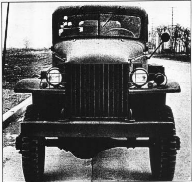
The late production third series CCKW in its most basic form. The early third series trucks looked just like the second series trucks. For this late model, the prominent identifying characteristics are: the wood-rimmed steering wheel, the semi-circular un-lead body seams at the lower corner of the windshield, the asymmetrical brush guard (without logo) and the factory installed blackout drive lamp. Not readily apparent, but it's there; the hood side panels show the screwhead that holds the bonding straps just above the fast louvre. Mar. 1943
