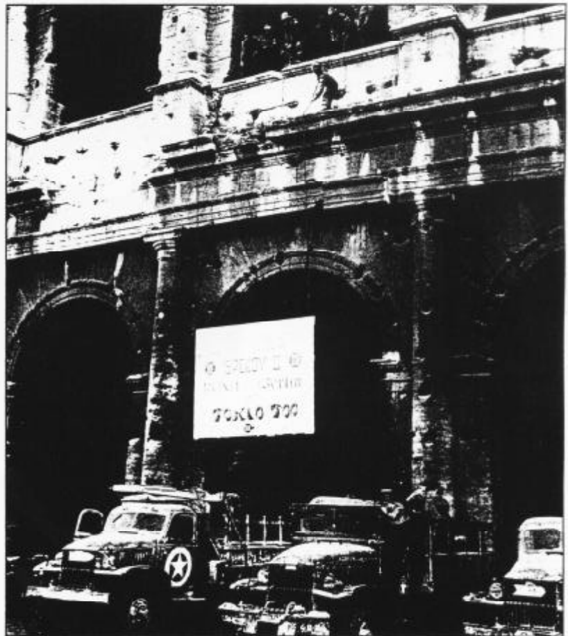
A pair of well worn, two-year old, third series CCKW's sit parked at the Coliseum in Rome. The closed cab 352 shows the most commonly used brush guard - the symmetrical one with logo, and field applied B.O. drive lamp. The early open cab 353 has the rare asymmetrical brush guard with the factory mounted B.O. drive lamp, and the GMC logo that was used on only about 10,000 trucks built early in 1943. They look like they have already been owned by a construction company. November 6, 1944 US Army Photo SC-313005
