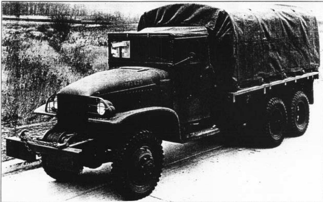
A real late fourth series truck. It still has the 1942/43 style wooden cargo bed, but it has the very late improved cab with the revised, late style large windowed doors, and the much tighter metal side rail reinforced top. Just barely visible you can see the shovel stowed on the running board. Yes, the small 2" regulation registration numbers finally appeared on CCKW's in mid 1943. January, 1944.
