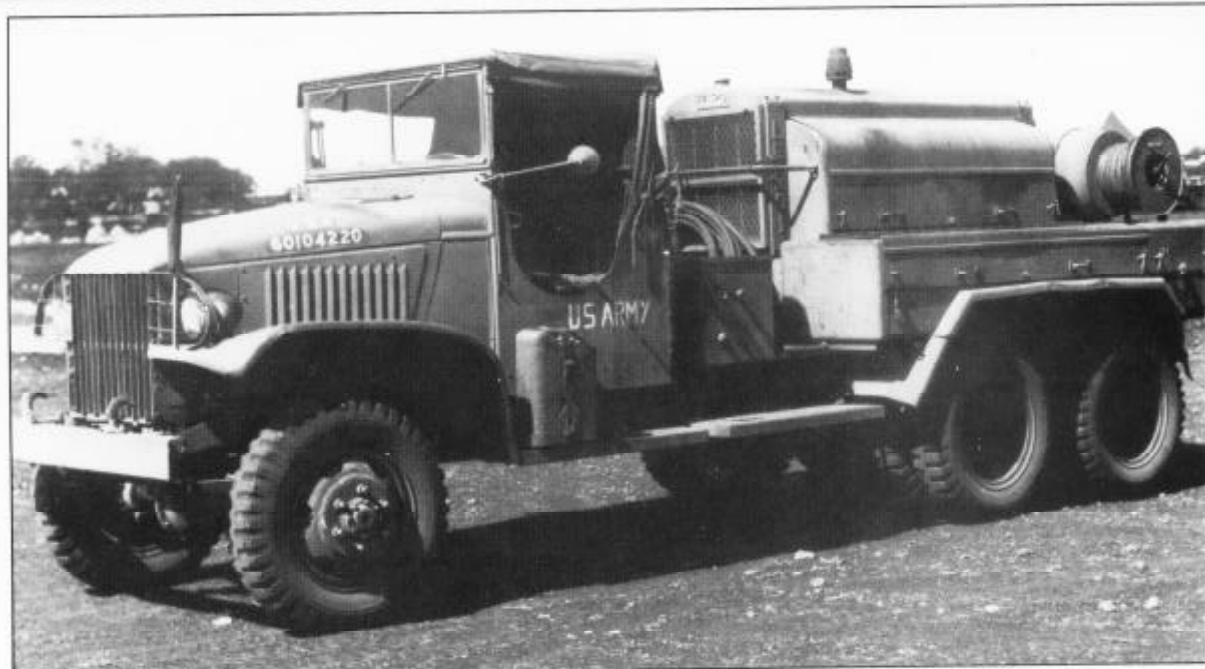
A perfectly average mid 1943 CCKW-353 Compressor Truck. It's late enough to have the gas can carriers, but not late enough to have the running board mounted pioneer tools or the late canvas. The top shown is the early one, without the metal side rail. The only options are: the unit badge and flag on the brushguard, and the kinked fenders. U.S. Army SC 380093
