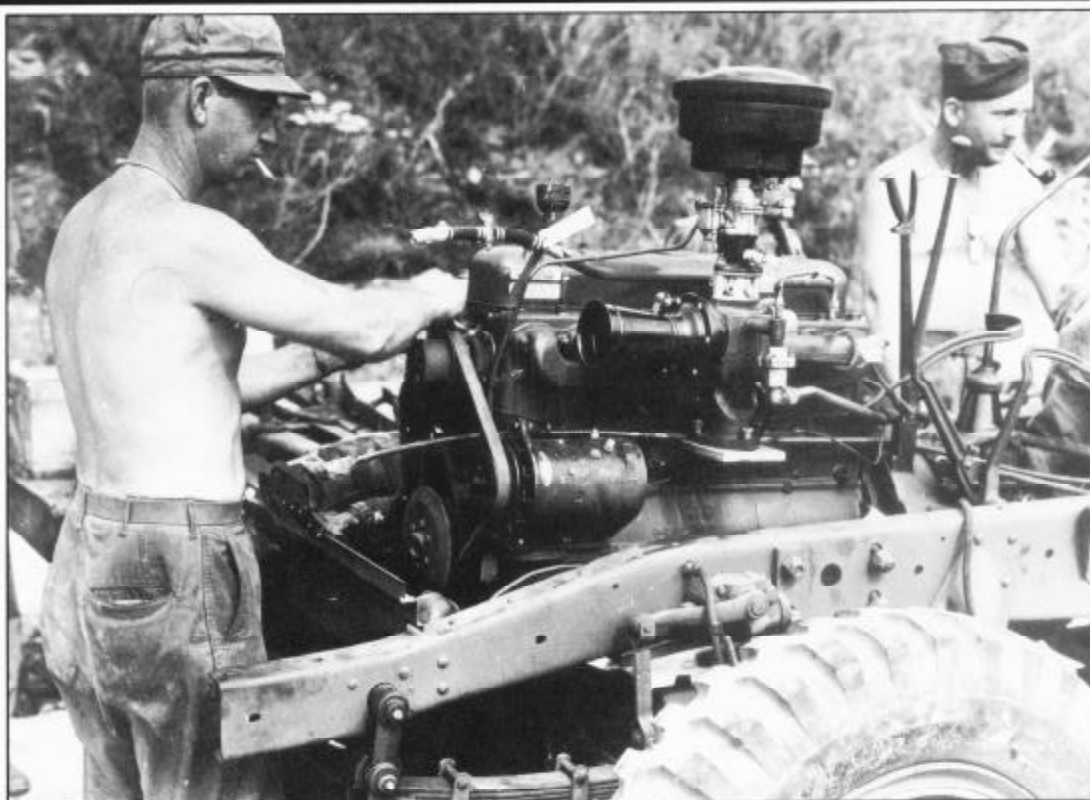
A field re-assembly of a crated GMC. Note all the shiny new parts and the octane rating and tappet setting on the valve cover. Date and place unknown.
