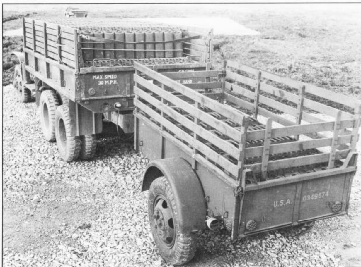
A rear view showing the late composite steel/wood cargobody. The load? Just over five tons of gas filled jerrycans. The steel bodied truck is matched to a steel-bodied one ton T-6 trailer. Dveon, England. Jan. 1944. U.S. Army SC 280107
