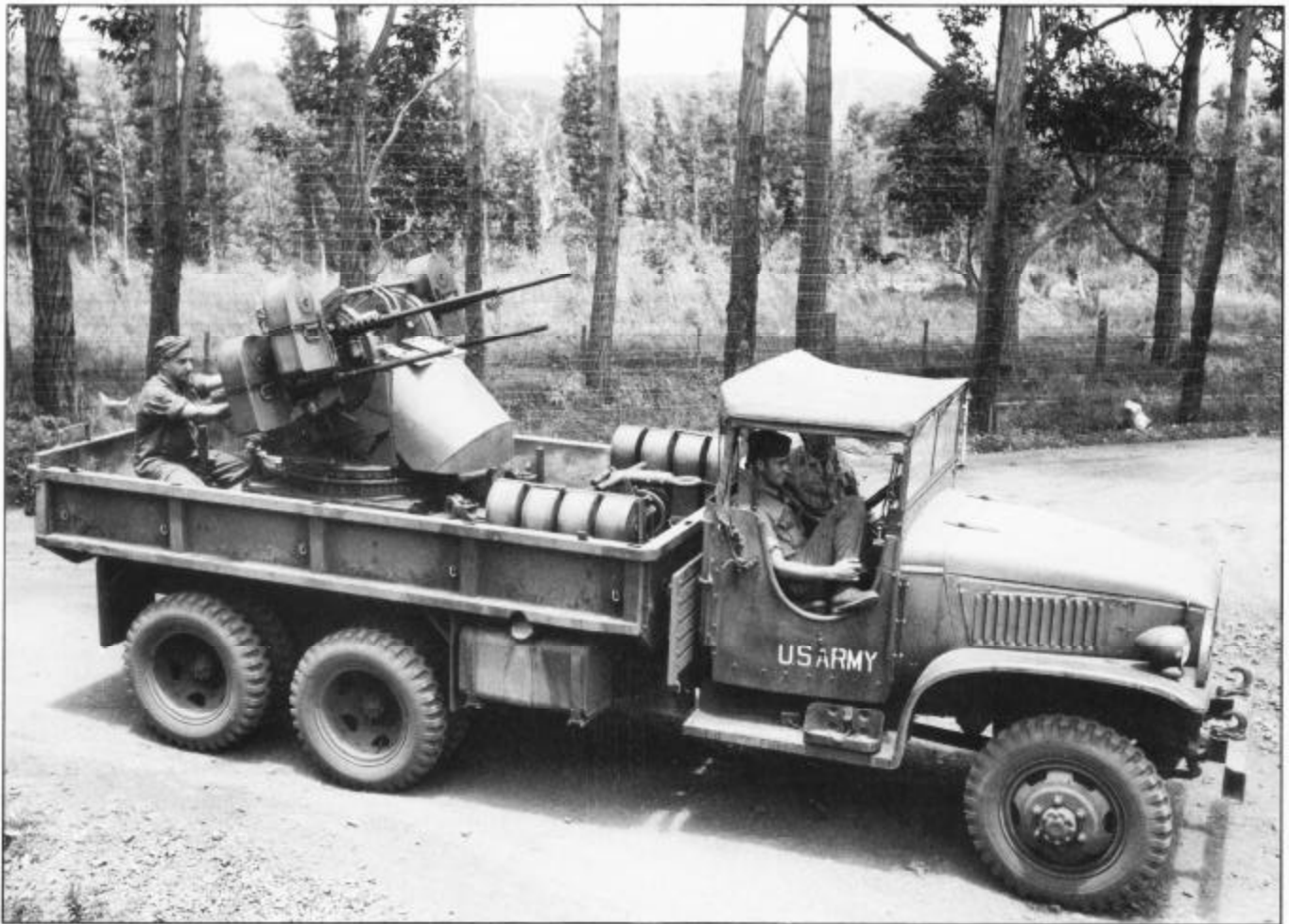
Externally, the only difference between the 1943 'Fourth-series' and the 1944 era 'Fifth-series' trucks, is that the cargo trucks used the late war developed composite steel/wood bed. Interestingly, no factory portraits of the late cargo body exist. This is the best available shot showing the bolted together steel bed, with the wooden floor. The metal reinforced edge, or side rail in the canvas top is most evident in this view. The quad .50 mount has to be the ultimate accessory for your 'Jimmy'.
