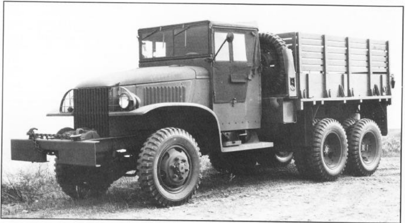
The definitive '6th-series CCKW - sort of. Actually it is a 5th-series truck photographed January, 1944. No photographs were taken of the CCKW after this date. No record can be found, even of the last one off the assembly line in August, 1945. Externally both the 5th and 6th-series trucks are identical. Only 6000 of the charismatic 352-B1's were ordered on the last contract. At this time it is not known if they had the all wood, or late bolted steel / wood body. 24 January, 1944
